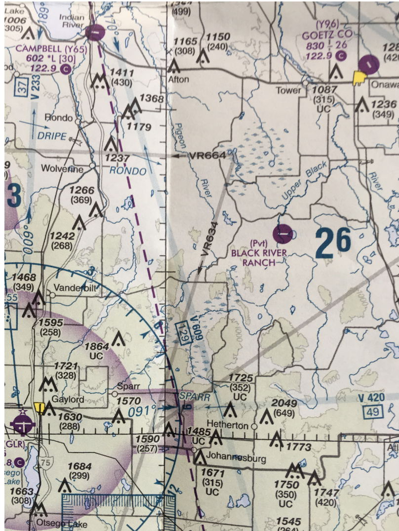
Low-level route VR634/664 shown on 2017 Michigan Aeronautical Chart goes east from Wolverine and turns sharply southwest over Dog Lake. The route is easiest to find looking just left of the words Black River Ranch in about the middle of this image.
